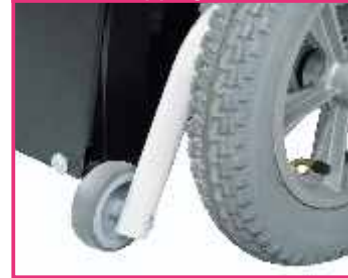
Ruedas anti-vuelco Anti-tipping wheels
